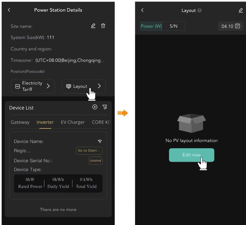
**Step 2:** Select the corresponding device to customize the component layout and then [Save] the settings. Afterwards, users can view the power and connection status of each component, and check the total power at the bottom.
