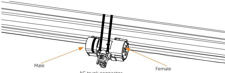
B) Plug the male terminal of AC trunk cable into the female terminal of AC trunk connector.
