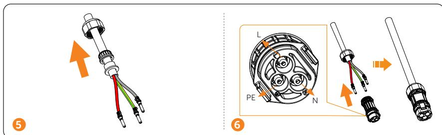
G) Insert the AC end cable-M to the last female connector of the AC trunk connector, and connect the other end of AC end cable-M to the distribution box (L, N and PE cables must be connected accordingly).
