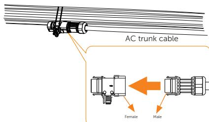
C) Band the AC trunk cable with cable ties. In order to better fix the AC cable, it is recommended to use more cable ties to band the AC cable.
