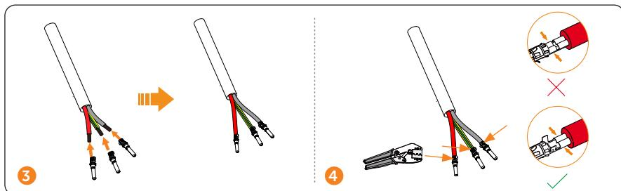
D) Thread part I, part II and part III into the AC end cable-M. Thread L, N and PE cables into the corresponding hole of part IV. Screw down part IV with part I.
